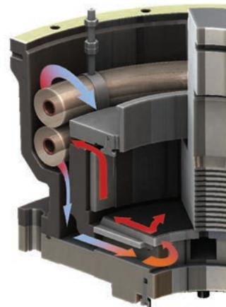
Oil circulation path during bearing operation
